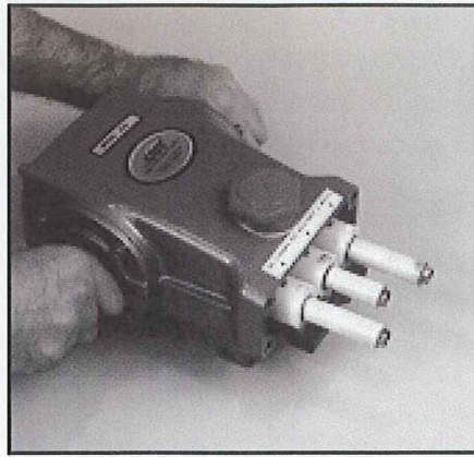
Proper Alignment of Ceramic Plungers for reassembly
